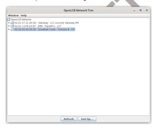
Open up this tree, and select "Open Configuration Dialog" in order to configure the device.
