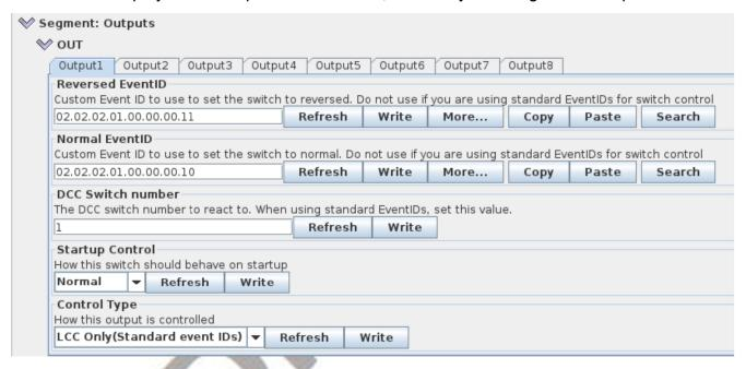
For most use cases, you may simply set the 'DCC Switch number' setting. For example, when the 'DCC Switch number' is set to '1' as shown in the picture above AND the 'Control Type' is set to 'LCC Only(Standard event IDs),' the SMTC-8 will automatically respond to the well-known event IDs 01.01.02.00.00.FF.00.09 and 01.01.02.00.00.FF.00.08.
